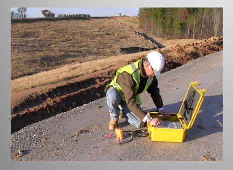
ASTM D7698 – 11 Standard Test Method for In-Place Estimation of Density and Water Content of Soil and Aggregate by Correlation with Complex Impedance
